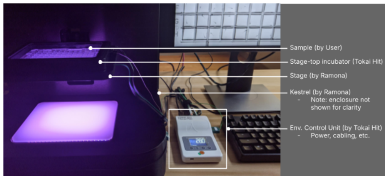
Fig 123: Close up view of the elements in the active control module.
