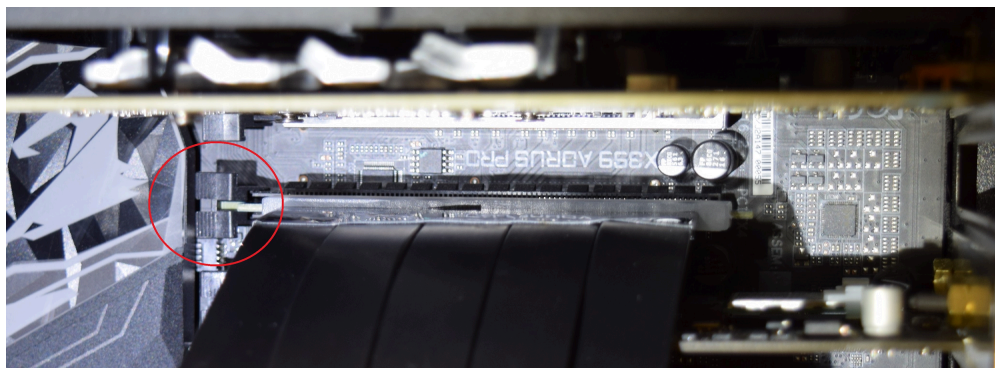
Figure 119: Connecting the PCIe Ribbon Cable to the MCAM workstation with connector lock highlighted.
