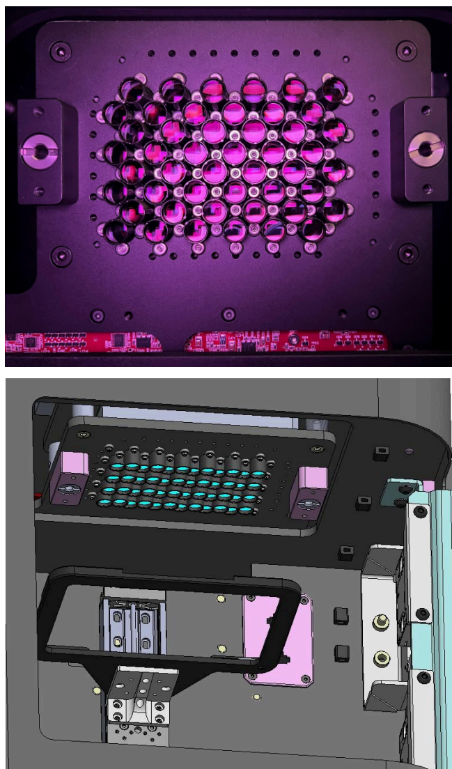
Fig 5: MCAM chamber upper interior surface with lens block
