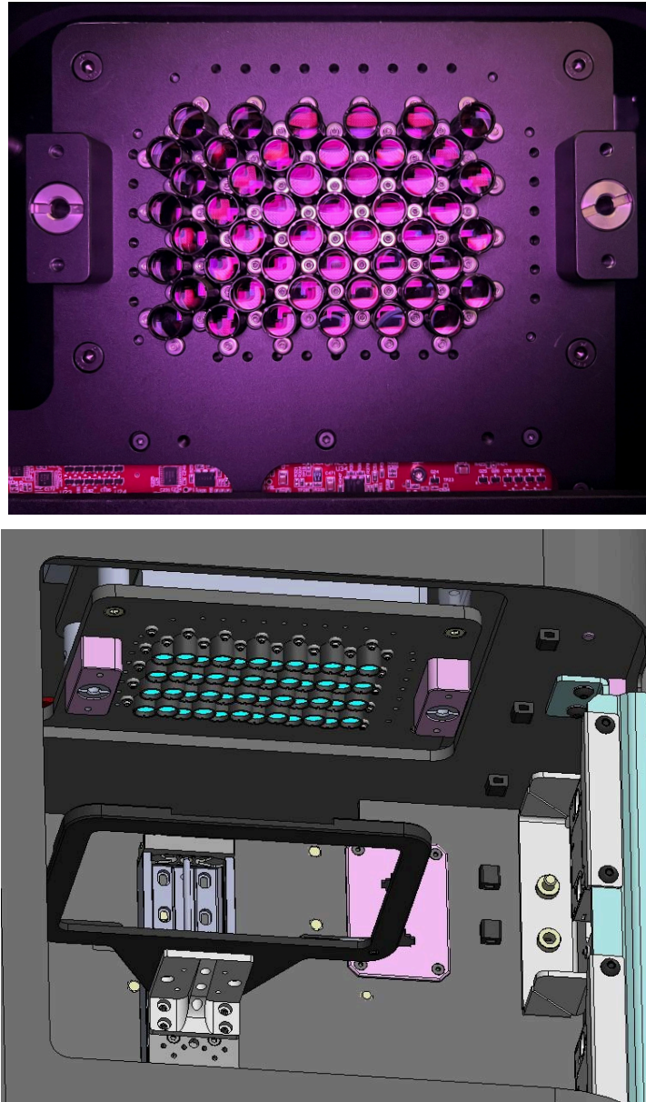
Fig 4: MCAM chamber upper interior surface with lens block
